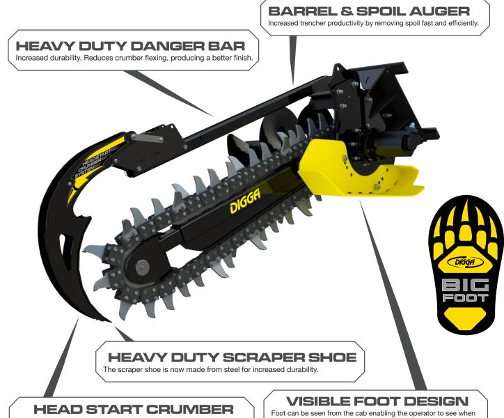
Start trenching with the crumber in the ground. Eliminates the need to step out of the machine once the trench is started, saving you time & money.
